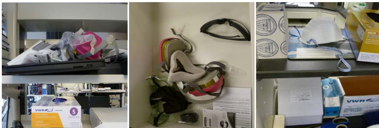
Figure B4. Respirators stored inappropriately in laboratories. Photos by NIOSH.
