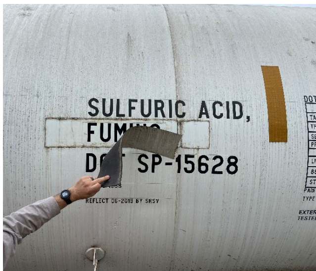
Figure B13. A magnet covering the word “fuming” on the label of the tank car. Photo by NIOSH.
