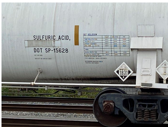
Figure B12. A tank car labeled “Sulfuric Acid” displaying a DOT placard with UN Number 1831 and the corrosive chemical pictogram. Photo by NIOSH.
