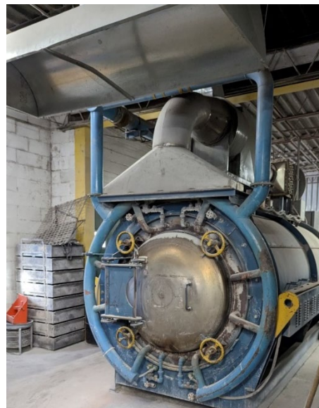
Figure B5. Two overhead exhaust hoods over the cylindrical retort furnace. Photo by NIOSH.
