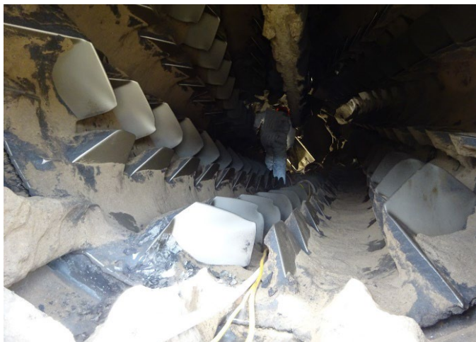
Figure A7. Worker chipping buildup off vanes inside mixing drum located within the yard. Photo by NIOSH.
