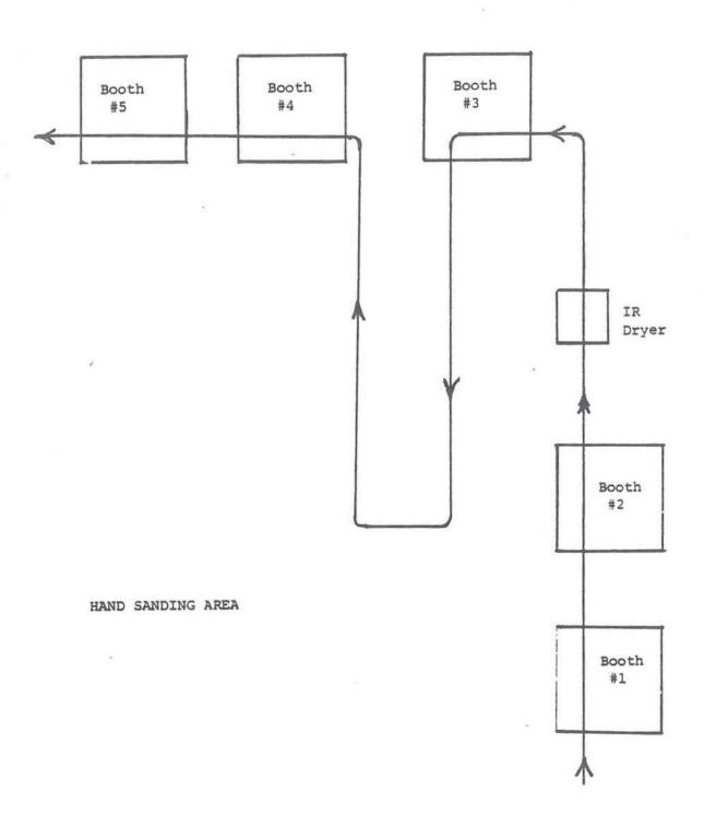
FIGURE 1: General Layout of the Finishing Area
