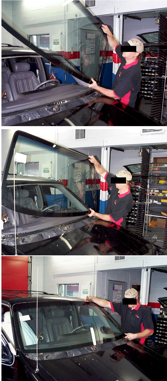
FIGURE 1. Installation of windshield
