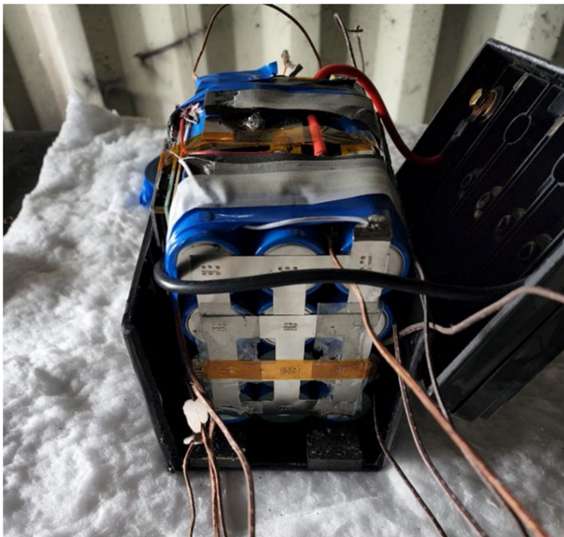
Fig. 2. LFP battery pack with thermocouples attached
