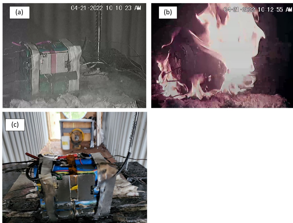
Fig. 6. Battery fire suppression using water mist. a Smoking of battery; b flame before suppression was on; c complete extinguishment
