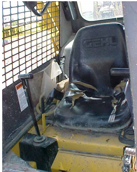
Photo 2. Position of safety bar following the incident.
