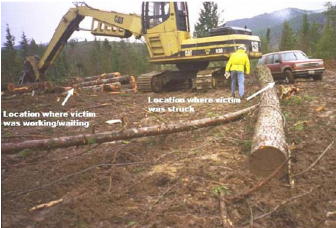
Photograph 3. The event site and log that struck the worker.
