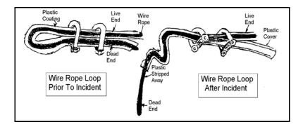
attached to the boatswain's chair support cable by two U-bolts and duct tape.
