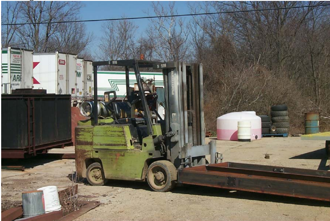
An example of how the fork truck was used to lift the metal plate. This plate is similar to the one that fell on the business owner.
