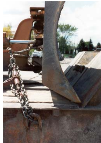
Figure 14. Proper attachment to "D" ring
