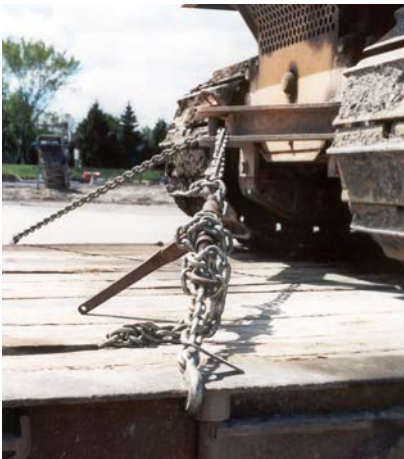
Figure 13. Improper attachment of loader to trailer bed
