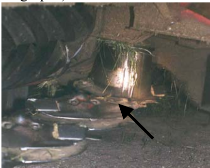
Figure 3 – Damaged Mower Disc
