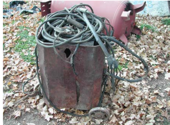
Figure 1- Overall Poor Welder Condition
