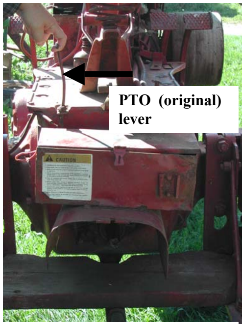
Figure 4. Original PTO engagement configuration
