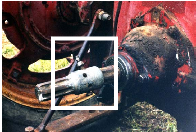
Figure 6. Unguarded PTO extension bolt
