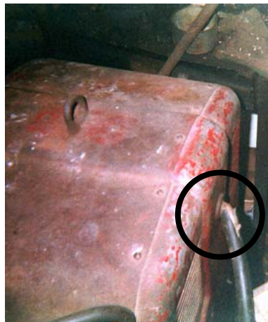
Figure 3. Damaged insulation on electrical cord
