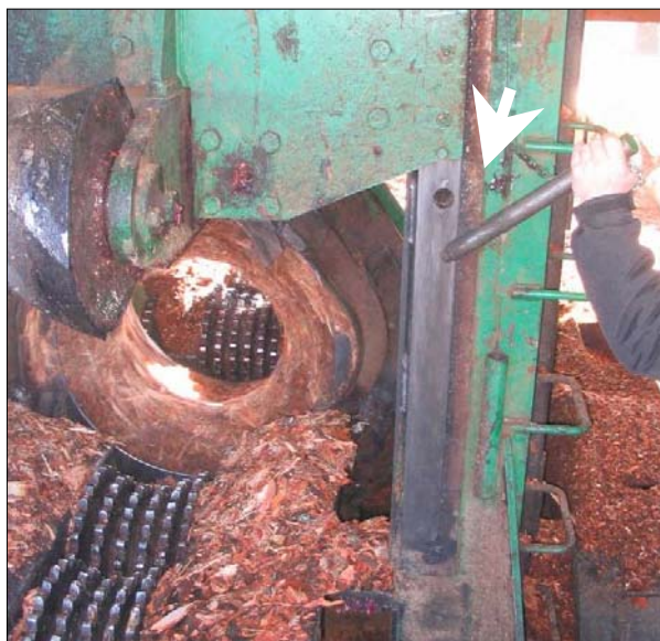
Intake of log debarking machine, showing one of two pins affixed to the frame of the machine by a chain. The pins can be inserted into designated slots to prevent the press roll from lowering. (see arrow)
