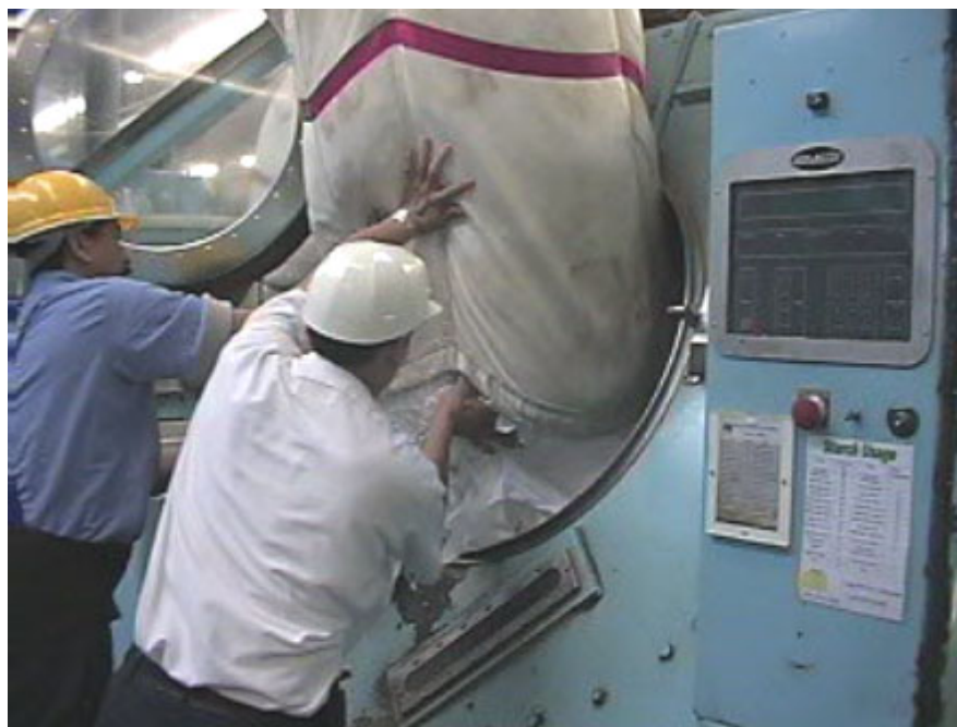
Exhibit #7. View of the laundry sling being unloaded into the industrial washing machine.
