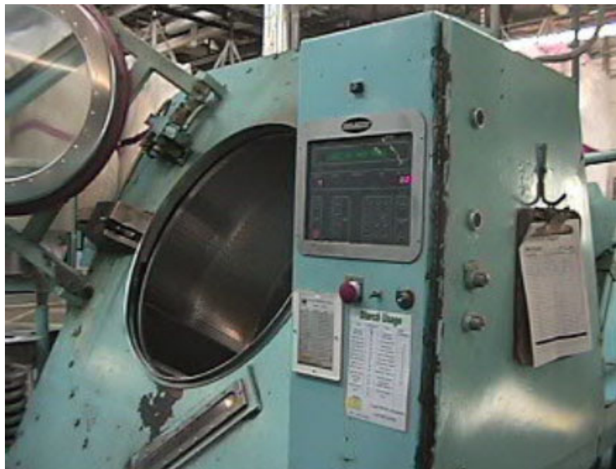
Exhibit #3. View of industrial washing machine in tilt position with loading door open.
