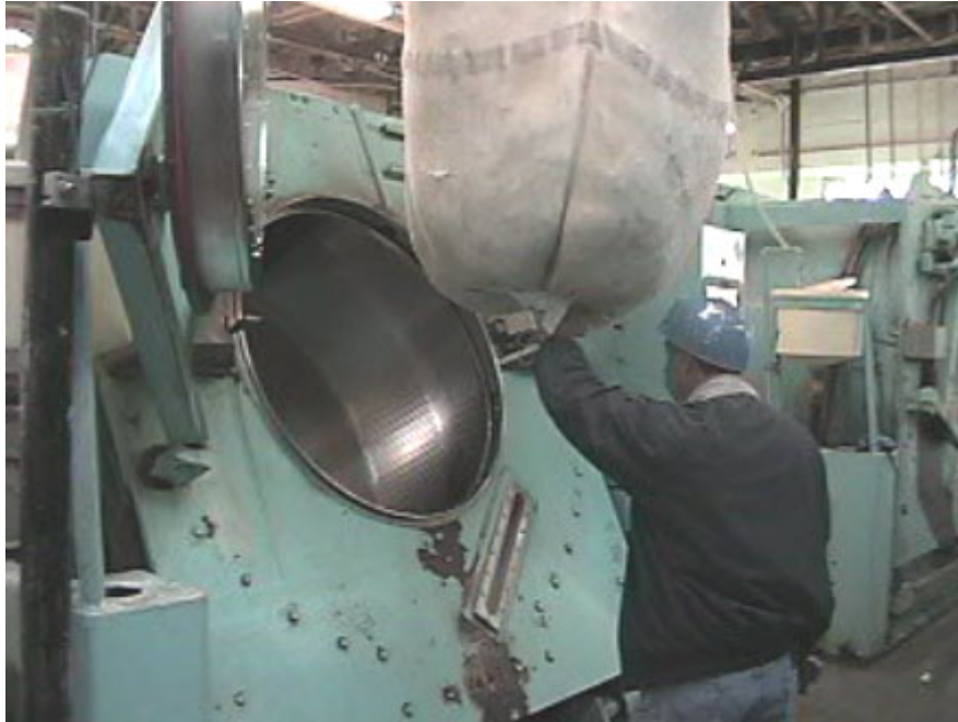
Exhibit #6. View of the laundry sling in front of the industrial washing machine.
