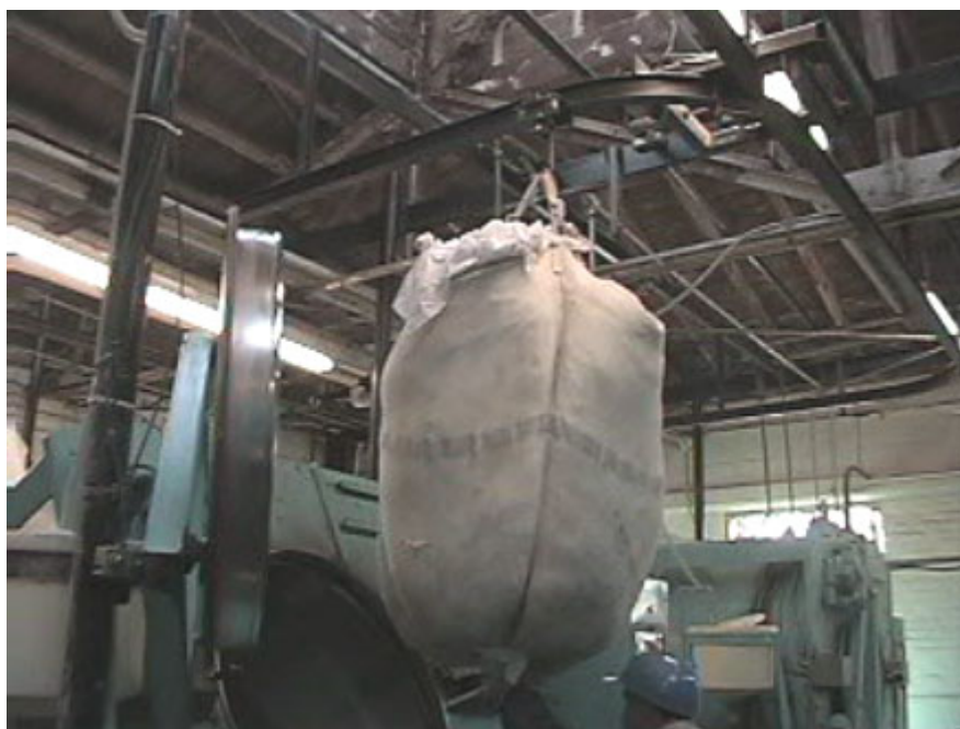
Exhibit #5. View of the laundry sling used to deliver laundry to the machine.
