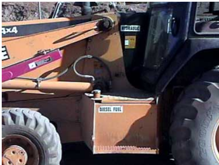
Exhibit #2 Close-up view of the step and handrail used by the victim.
