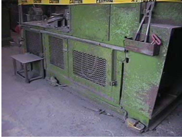
Exhibit #8 View of the inoperative safety bar wired to the machine.
