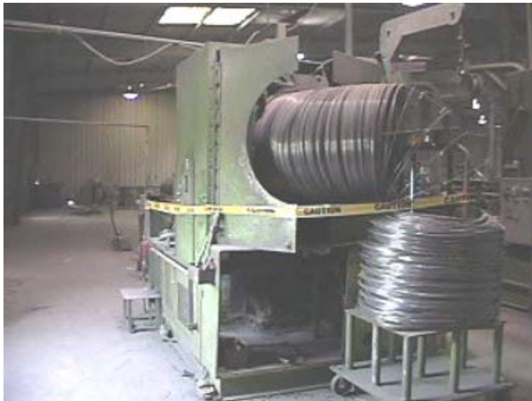
Exhibit #2 View of the wire pulling machine and the wire holding device.
