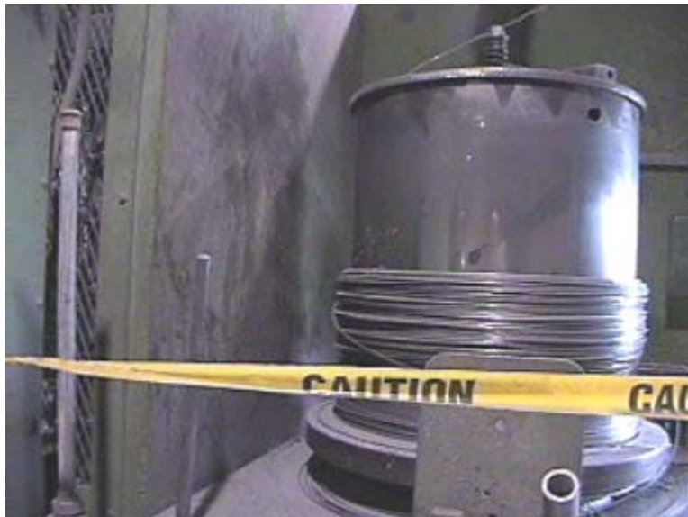
Exhibit #4 View of the rotating drum showing the area where the victim got pulled into.
