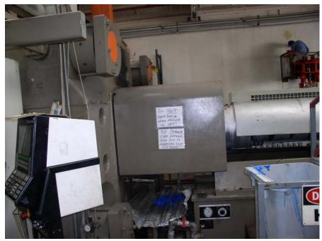
03CA004 Exhibit #5 View of the injector mold with protective shield in place.
