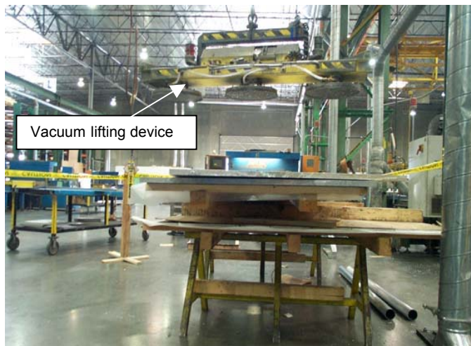
Exhibit 2. The three-cup vacuum lifting device suspended above the aluminum plates.
