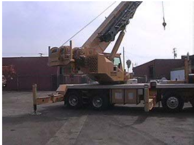
Exhibit 2. The truck-mounted crane rotating into position, depicting the blind spot for the operator.
