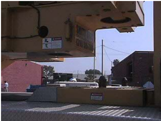
Exhibit 3. The base where counterweights are placed in order to be attached to the crane.
