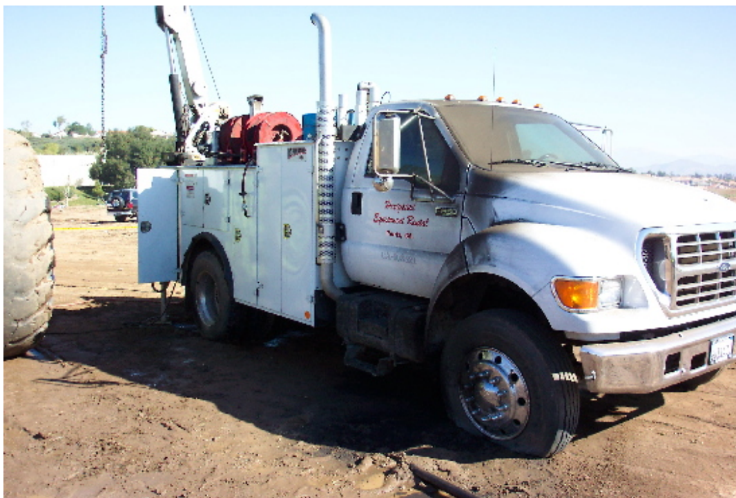
Exhibit 3. The victims' truck with the boom that made contact with the high voltage lines.
