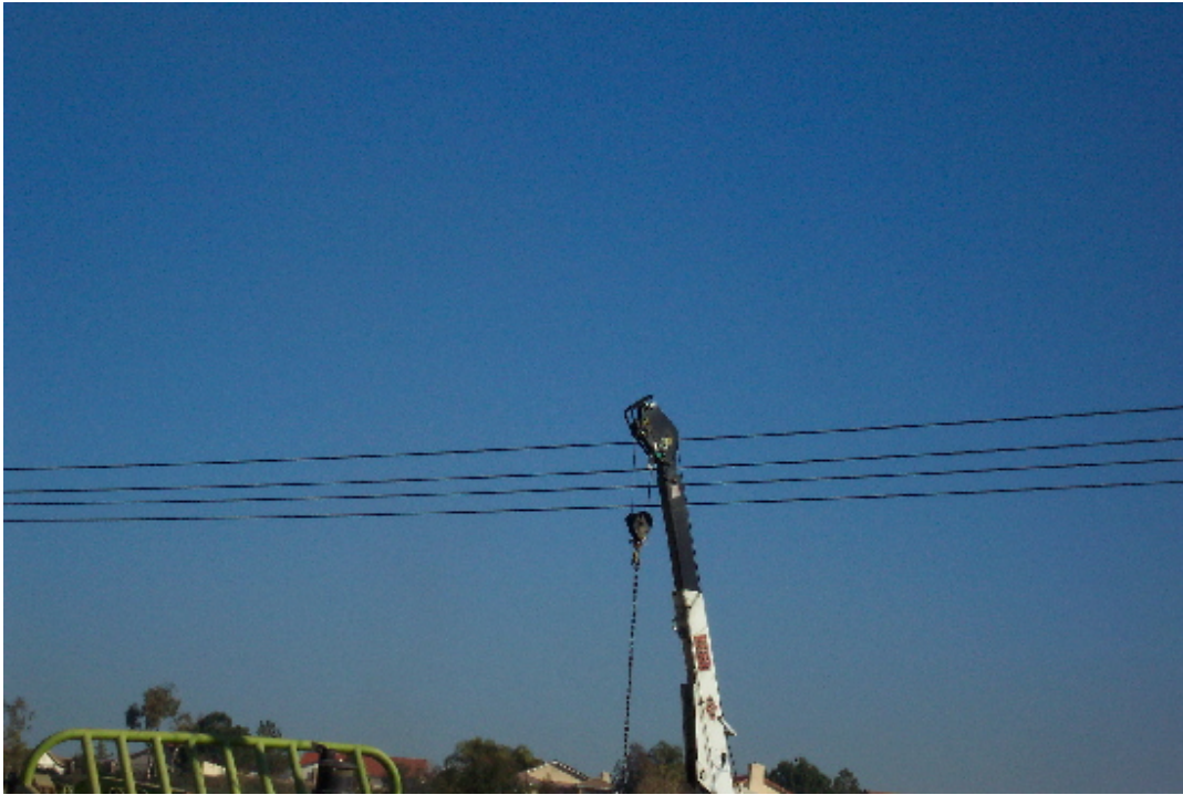
Exhibit 2. A picture of the incident scene with the crane boom still in contact with the high voltage electric lines.
