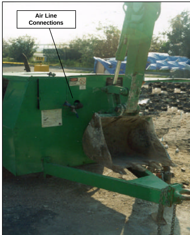
Photo 3. Bucket of Mini-Excavator and Air Compressor. One of the air lines was pulled free of its connection to the air compressor. When the bystander and the victim entered the area to investigate, they were momentarily pinned between the mini-excavator bucket and the air compressor.
