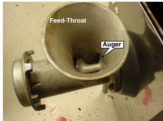
Photo 4. Grinder Housing, Auger, and Feed-Throat
