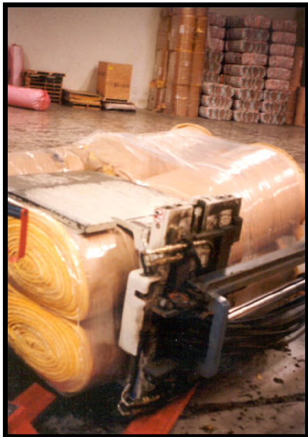
Photo 2. This photo illustrates the clamp attached to the forklift mast which is used to grasp and hold the rolls of fiberglass in place.
