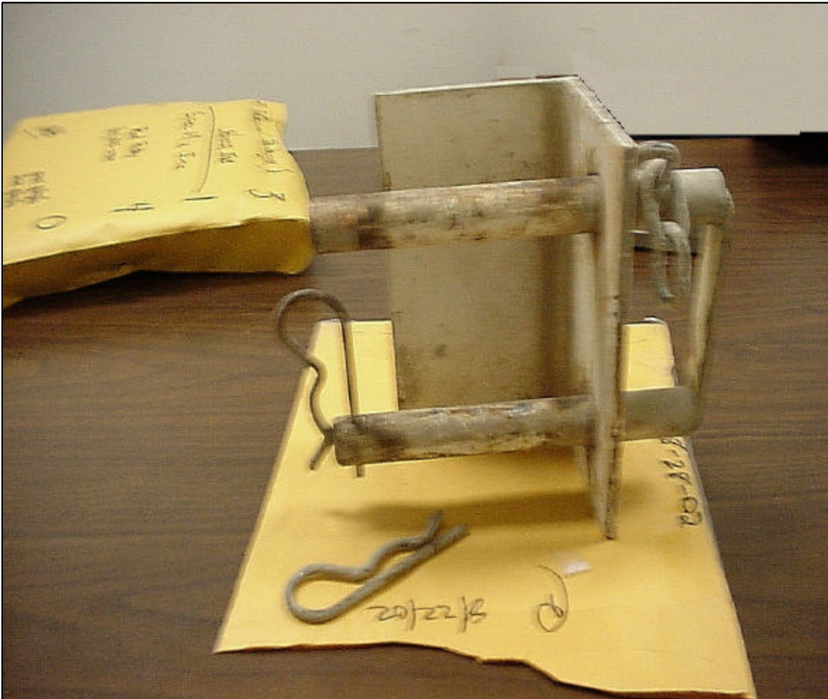
Photo 1. This photo illustrates the two-pronged hitch pin used to hold the silo legs in place.
