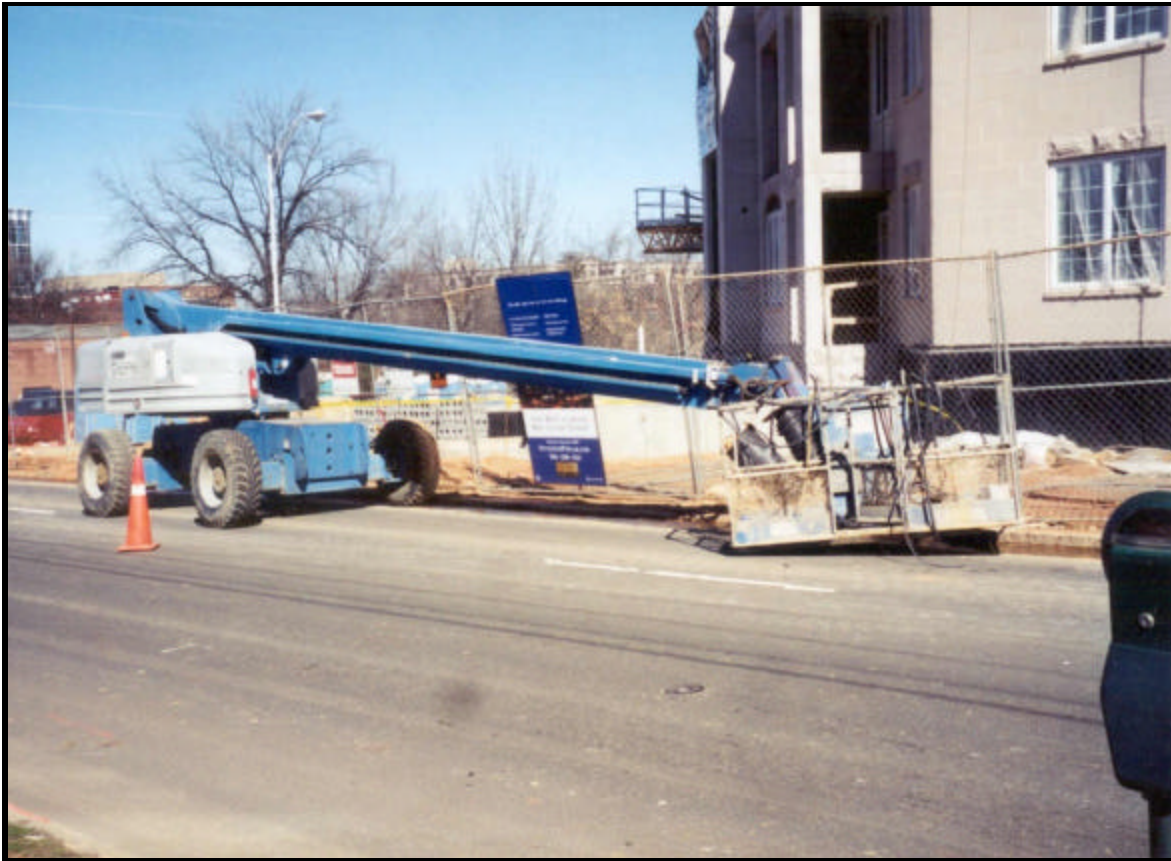
Photo 4. This photograph is of the boom-supported aerial platform which should have been used for the task performed in the incident. This photo illustrates that the traffic lane would have had to be closed when the equipment was in use
