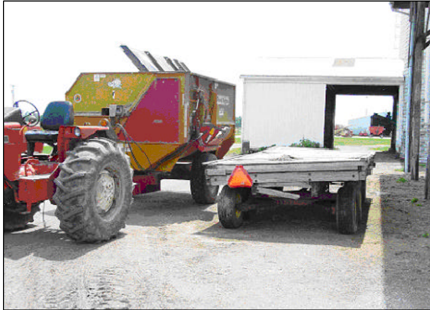
Photo 3. This photograph depicts the hay wagon that is used in the process of loading the feed grinder-mixer. Note: the hay wagon is normally positioned on the other side of the machine for loading purposes
