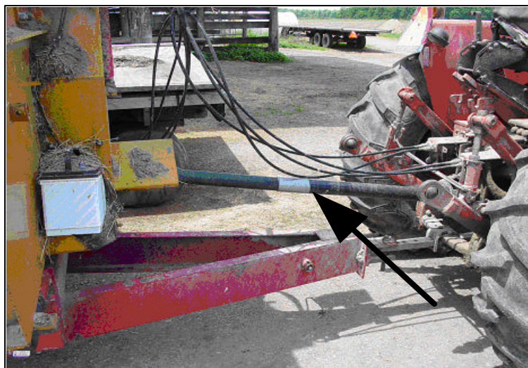
Photo 1. Depicts the power-take-off shaft engaging the feed mixer-grinder from the rear of the tractor
