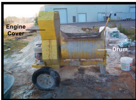
Photo 1. Mixer with drum guard fully open
