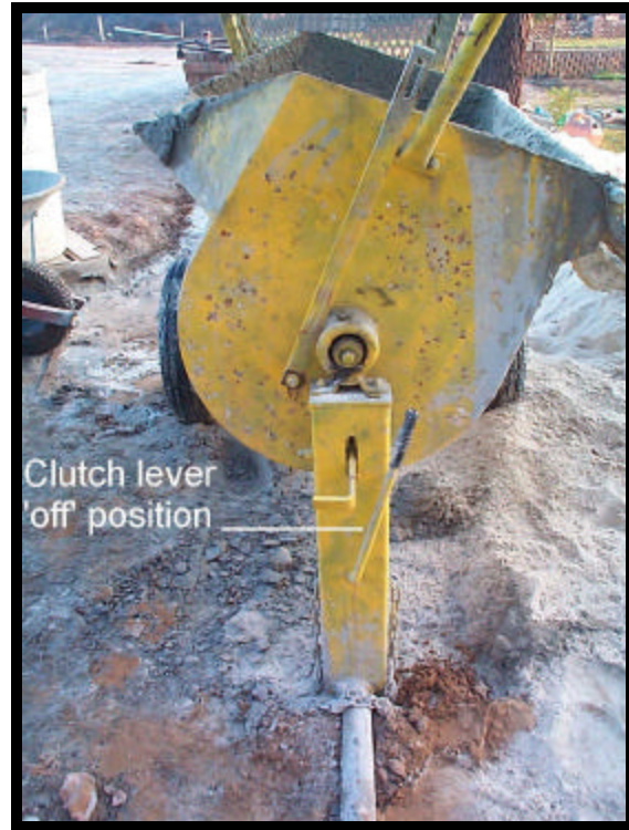
Photo 4. Guard off, clutch in the 'off' position
