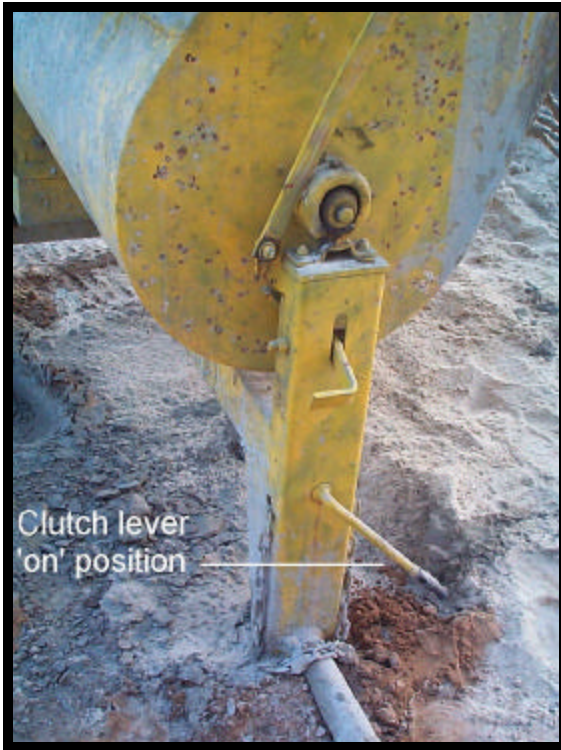
Photo 3. Clutch in the 'on' position, paddles rotating
