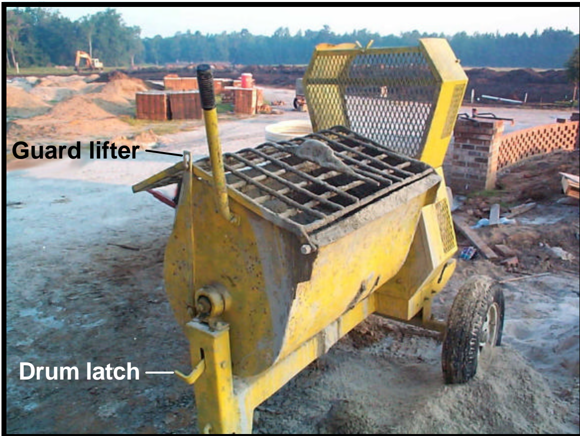
Photo 2. Guard lifter attached with guard in closed position
