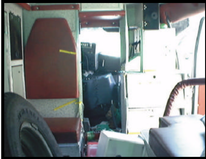
Photo 5. View of patient compartment after the vehicle was recovered from site. Patient contacted seat back at upper location, cot contacted at lower location. Contact indicated by yellow markers (source, National Automotive Sampling System)
