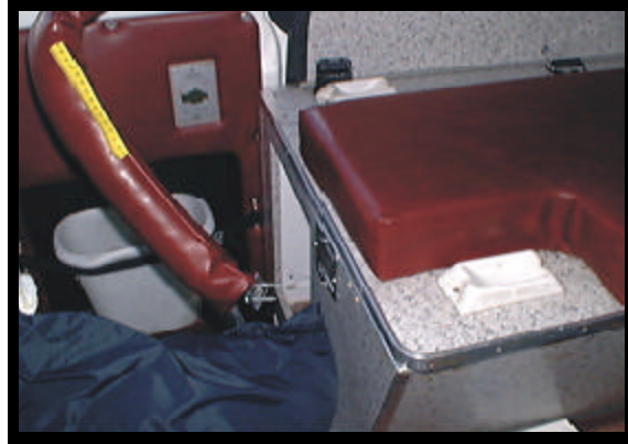
Photo 3. Victim contacted and broke a handrail at forward end of squad bench (source, National Automotive Sampling System)
