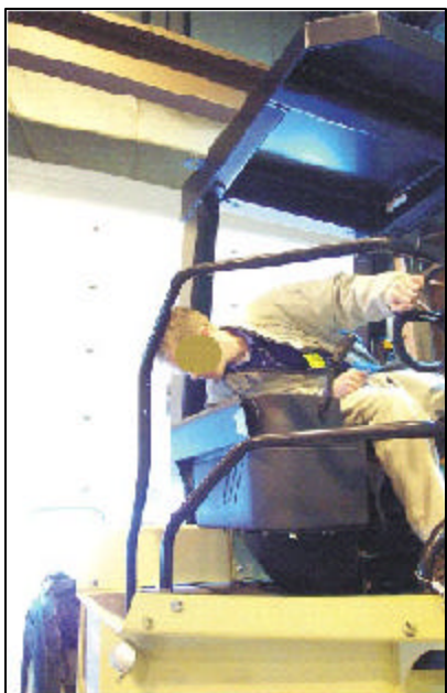
Photo 2. Seat belted operator on a compactor similar to that involved in the incident
