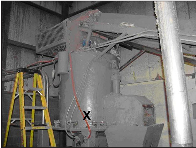
Photo 1. This photo illustrates the Densifier in which fatality occurred. The rotor blade is located inside the Densifier and its approximate location is marked with an X. [Photograph courtesy of TDLWD].
