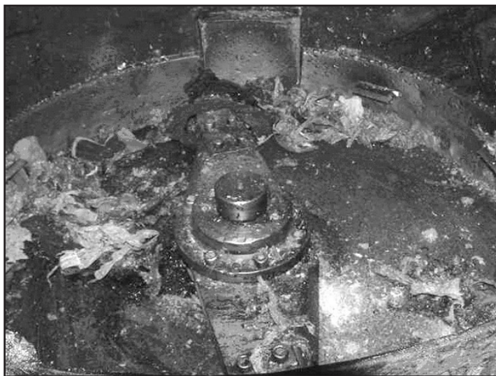
Rotor blade located inside and at the bottom of the Densifier. [Photograph courtesy of TDLWD]
