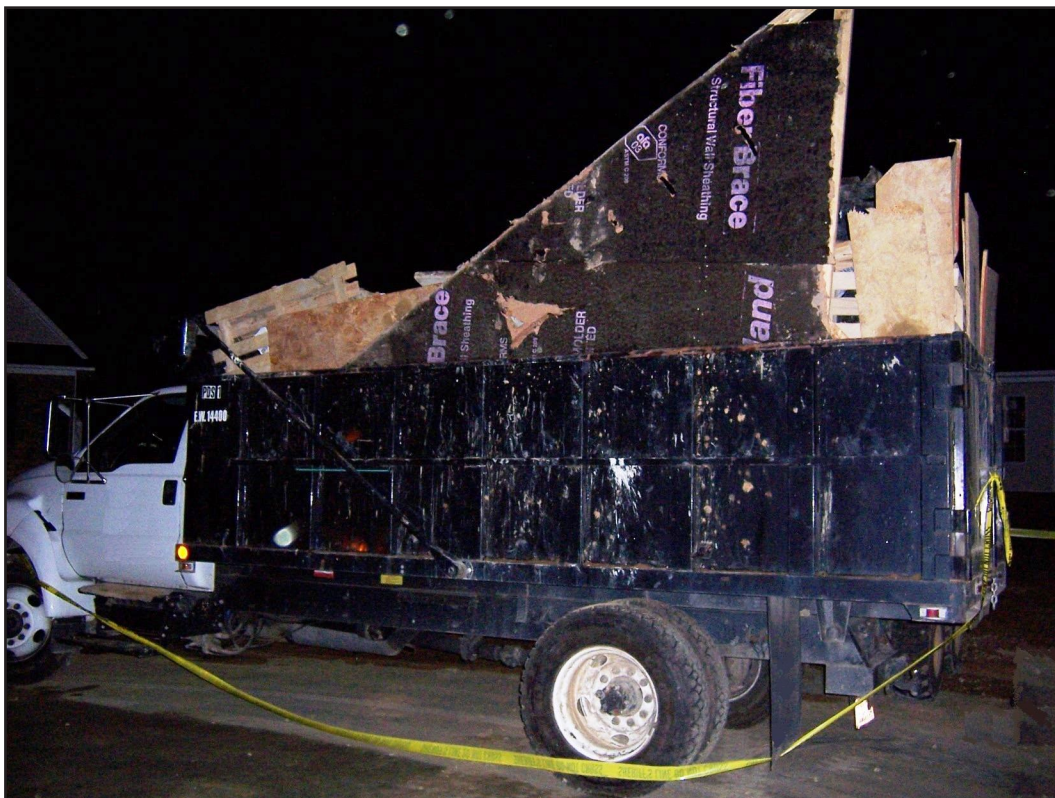
Photo 1. This photograph illustrates the trash truck used on the day of the incident. Scrap plywood pieces had been used to extend the truck bed height an additional 24 inches. [Photograph courtesy of NCOSH].
