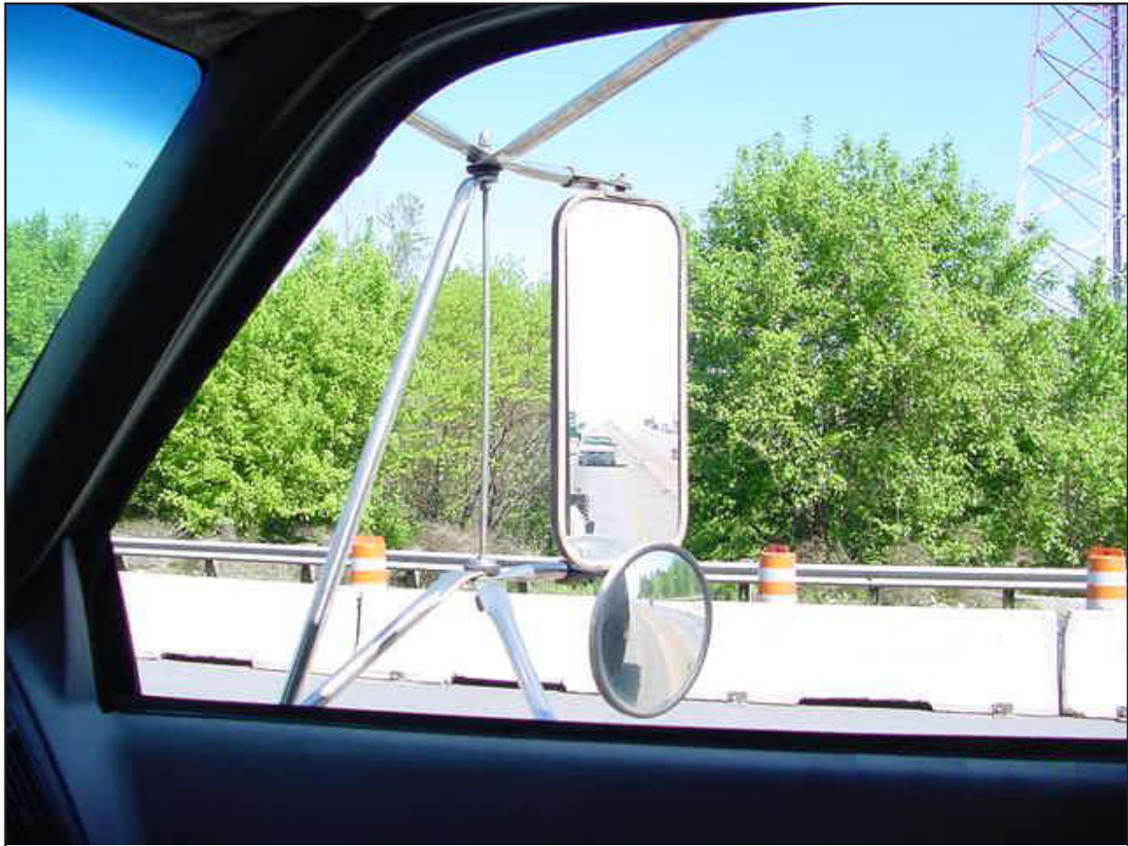
Photo 3. Photo of the mirrors mounted on each door of the dump truck. [Photograph courtesy of the NCOSHA].
