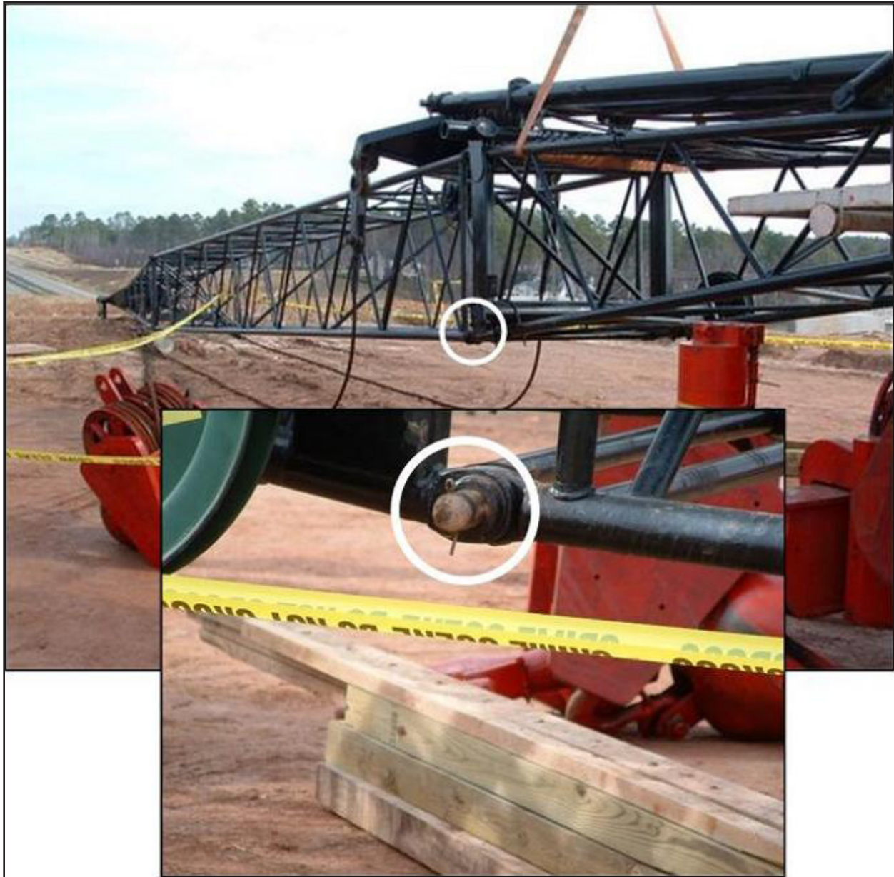
Photo 3. This photograph illustrates a close up of the location where the victim was struck by the boom. The 4x4's shown on the photograph were brought to the site and used to pry the boom up as it was lifted by the second crane. The pin is marked with a circle and was one of two lower pins removed. The two lower pins had been replaced during rescue efforts. An insert shows a larger illustration of the pin. [Photograph courtesy of NCOSHA].
