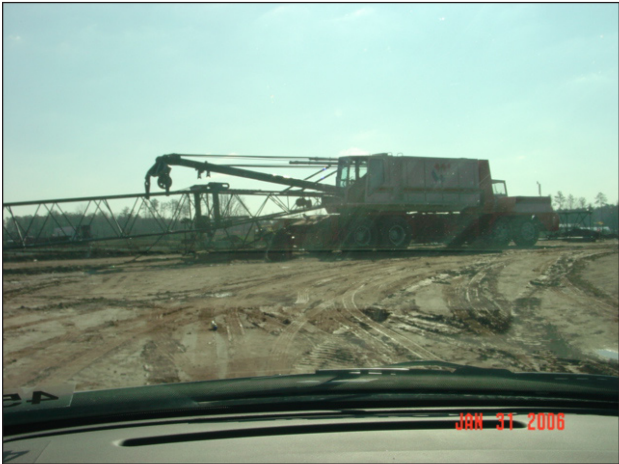
Photo 1. This photograph illustrates the truck-mounted lattice boom crane that was involved in the incident [Photograph courtesy of NCOSHA]
