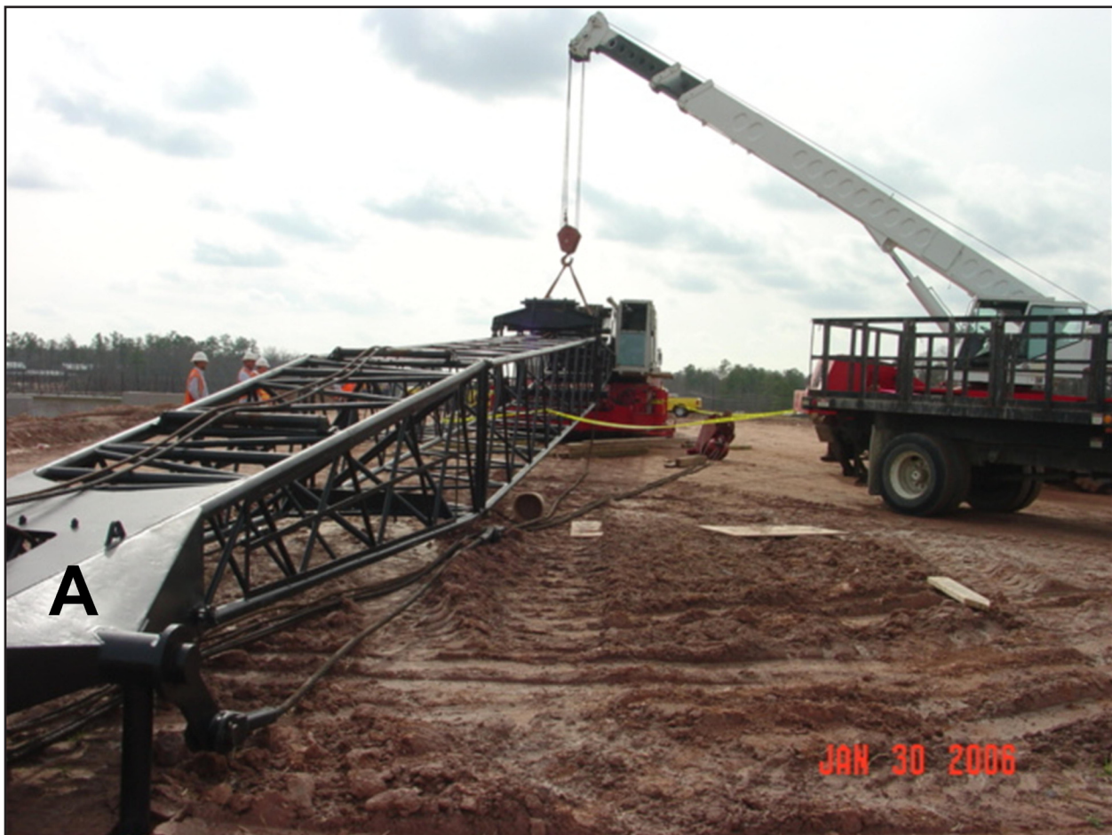
Photo 2. This photograph illustrates the peak of the lattice boom (A) after it had been lowered to the ground [Photograph courtesy of NCOSHA].
