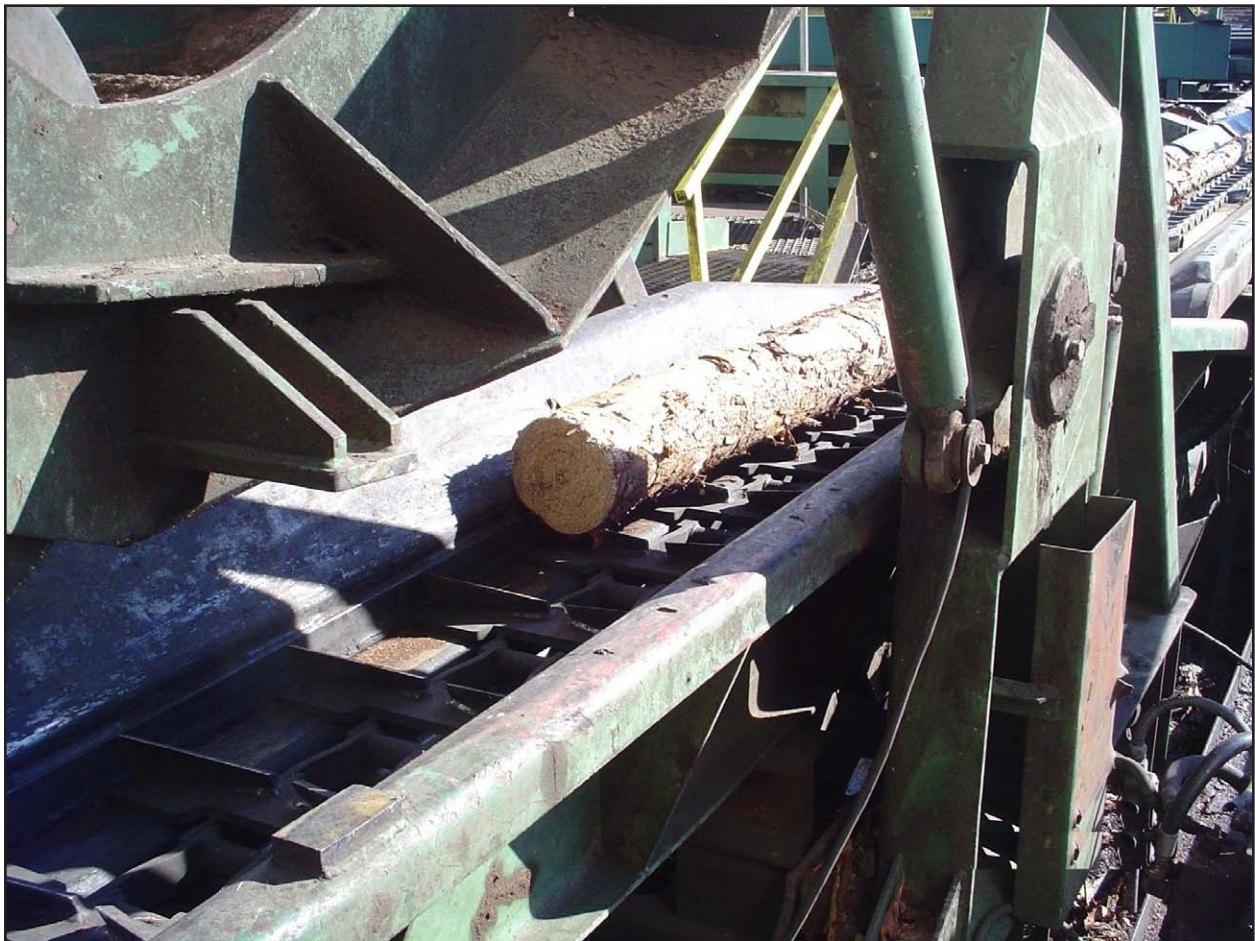
Photo 1: This photograph illustrates the conveyor moving logs into the south debarker [photo courtesy of SCOSHA].
