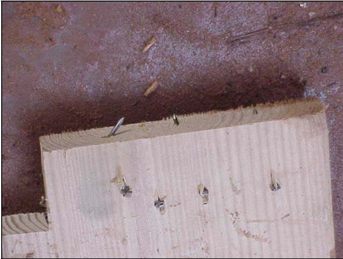
Photo 3: This photo illustrates the 8d nail placement on one end of the joist that failed (Photo courtesy of NCDOL/OSH).
