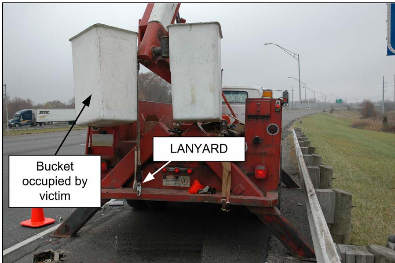
Photo 3. Photo of upper boom showing dual buckets and lanyard (photo courtesy of OSHA).
