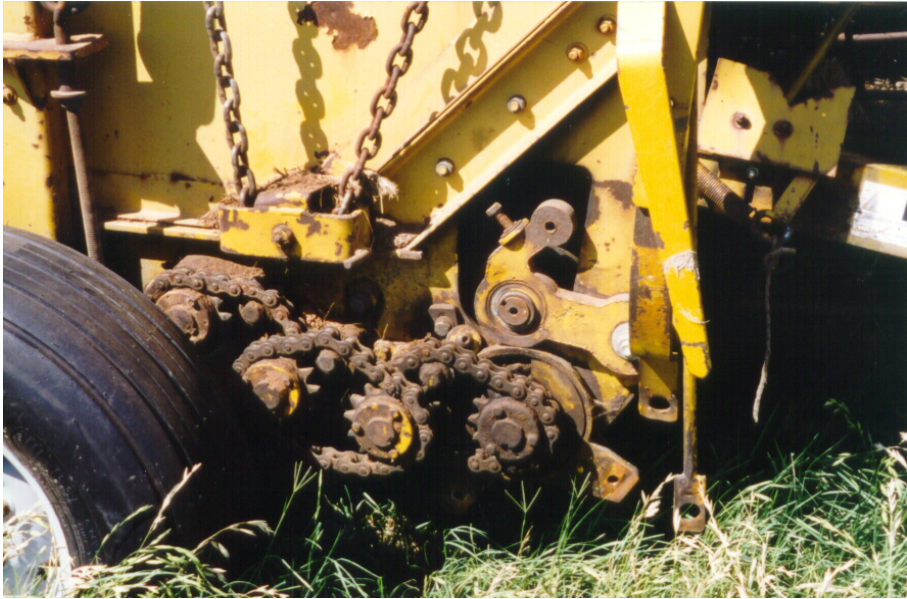
Figure 2. Area shown is the area in which the fire started. The protective shields were removed after the fire.
