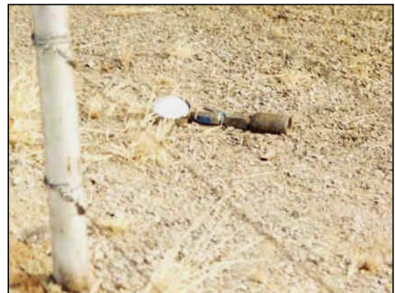
Figure 2. Bull plug, needle valve and gauge assembly
