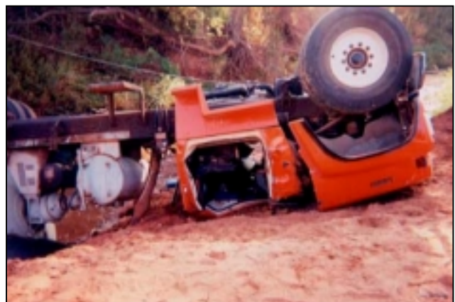
Figure 2. Close View of Crushed Truck Cab
