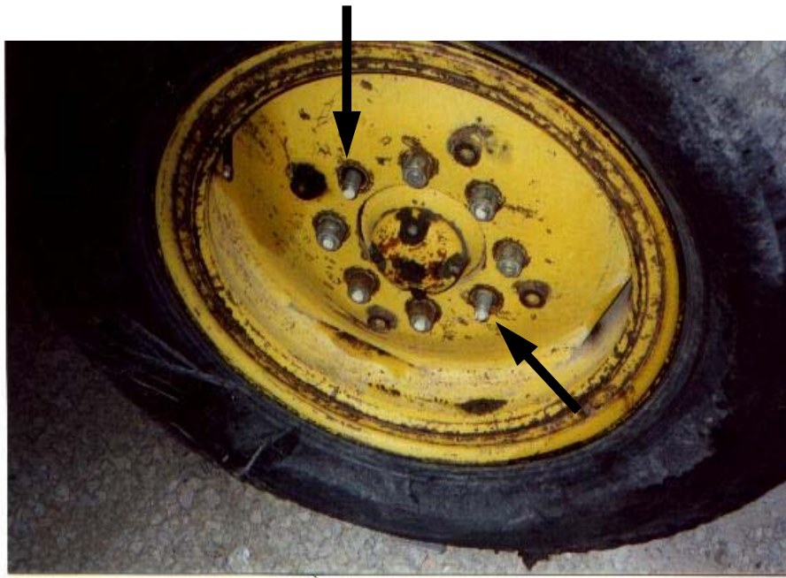
Photo #11. Left rear-steering wheel with two missing lug nuts.
