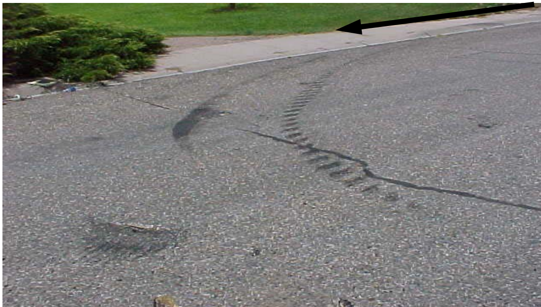
Photo #4. Tire skid marks left after equipment contacted concrete curve and veered to the left, before completing a 3/4 roll. Arrow notes direction of equipment travel.
