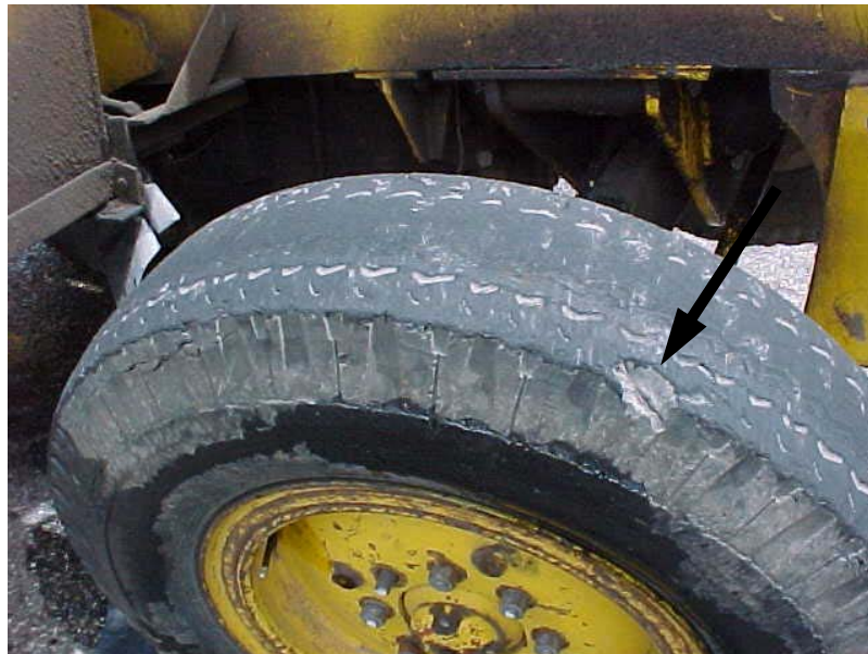
Photo #12. Left rear-steer wheel. Note the large chunk of rubber and most tread missing.
