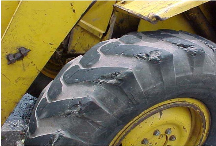
Photo #9. Left front-drive tire. Note missing tread and chunks of rubber.
