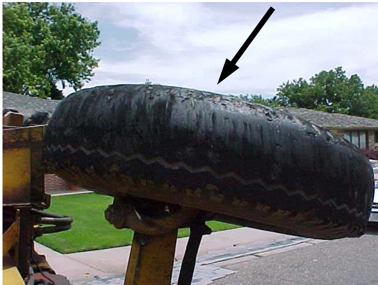
Photo #14. Right rear-steer tire showing missing tread and chunks of rubber missing from outside of tire.
