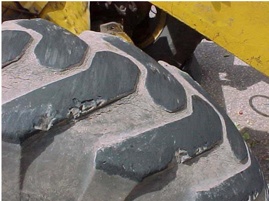
Photo #10. Right front-drive tire. Note missing tread and chunks of rubber.
