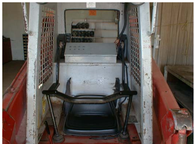
Figure 2. View of cab with seatbelts and restraint bar.
