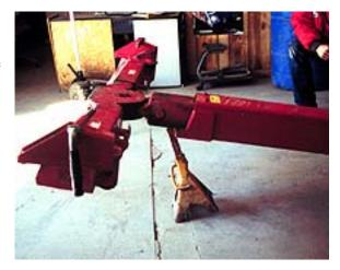
The tow truck was not damaged in the accident, however the truck was sold since its owner was friends of both men and he did not wish to keep the truck any longer. During our visit, he demonstrated the operation of a similar 6-way stinger. During demonstrations, placing the jack stand under a tilted stinger bar easily caused the stand to slip backwards, causing the tow truck to fall to the ground.
