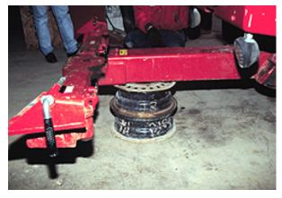
chocked. Demonstrations using a similar jack stand and similar stinger position showed that very little force or forward movement is required for the stinger to slip off the jack stand. Substantial supports, designed and rated for the type of vehicle, should be used when working under raised vehicles.
