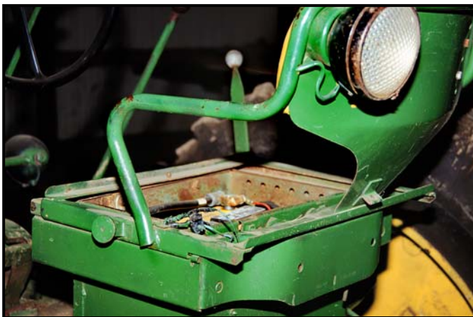
Photo 4 -- View of left side of seat, showing sliding track and armrests welded to the seat edge.
