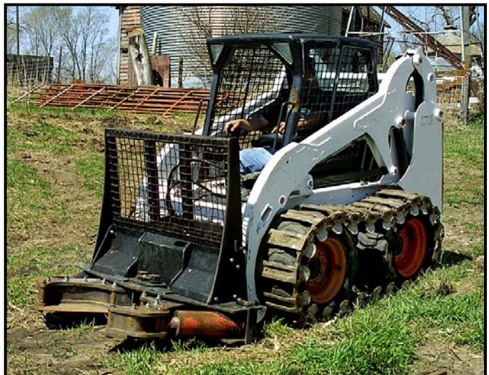
Photo 1 - Side / front view of loader with shear attachment.
