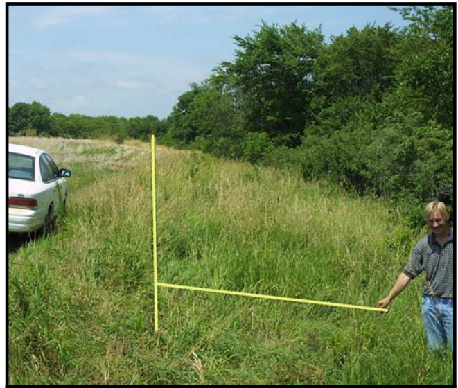
Photo 5 – Site of the overturn showing the location of the post and the downward ground slope of 8 degrees.
