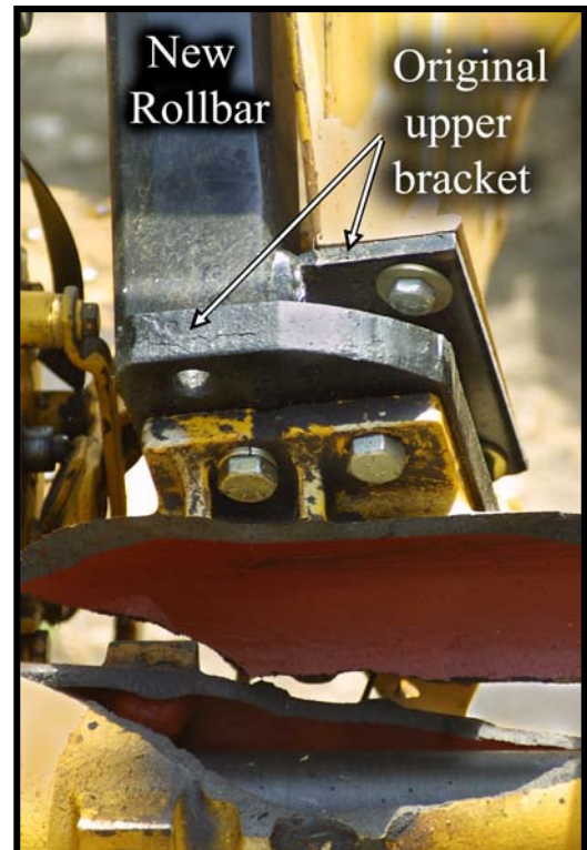
Photo 3 – Close-up view of right axle showing construction of rollbar and its attachment to the axle housing with short bolts. This also shows the original ROPS upper bracket with fender attachment, repainted to look new (refer to Diagram).
