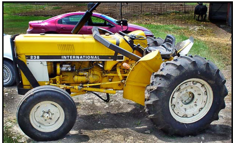
Photo 1 – Side view of tractor showing rollbar collapsed forward.
