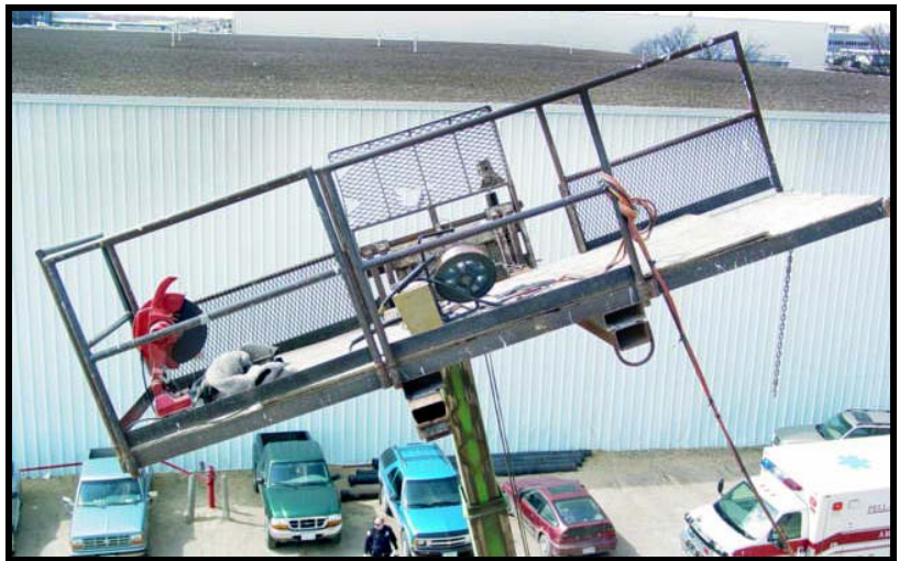
Photo 4 – View from the firefighter's ladder, showing details of the personnel platform, the tools onboard, the unprotected end, and the welded steel channels for the forks.
