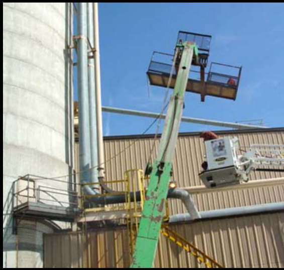
Photo 2 – Shot from the rear of the machine, showing the platform tilted far to the right.
