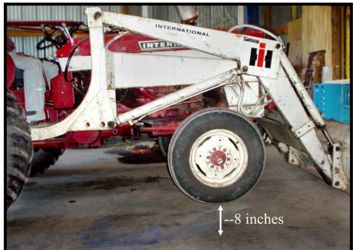
Photo 3 – Right side view of tractor with front bucket powered down to raise the front wheels off the floor.
